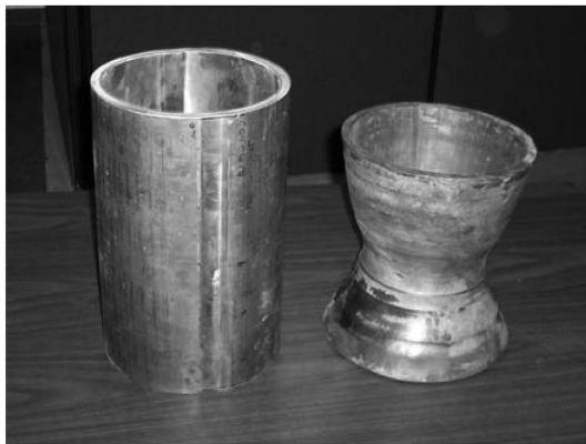
Fig. 17 Spun-formed liner before finish machining.
