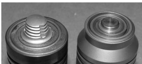
Fig. 13 Pin tools used for welding 1.27-cm (0.5-in.) thick GRCop-84; tack tool on the right, full-penetration tool on the left.
