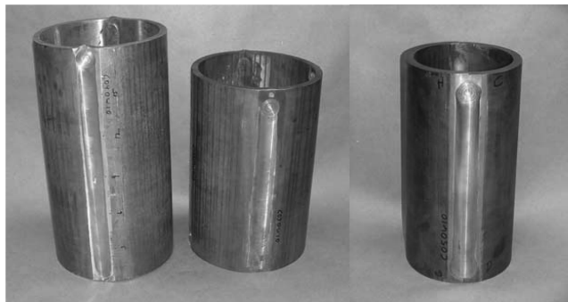
Fig. 14 Cylinders completed after welding.
